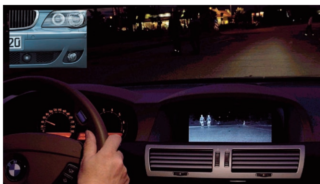
Figure 8. Night-vision scene obtained from an IR cameras that are used in the car-driving assistance system of BMW cars.
